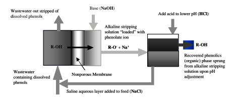
The MARS process recovers organic compounds which possess acid or base functionality (organic acids and bases, AAB) by extracting them across a non-porous membrane and concentrating them as ionised salts prior to recovery through pH adjustment. The process is thus able to recover and reuse materials which in most other technologies, such as biodegradation, are destroyed. Research areas include:
